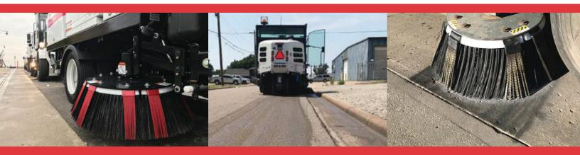
The Piranha is a universal attachment which supports the gutter broom. This revolutionary attachment clears the gap between asphalt and the concrete curb. It is capable of attacking weeds at the roots and clearing away stubborn weed seeds. The Piranha's durable but light segments are designed to reduce stress on the hydraulics by reducing gutter brush friction. This will not only result in less stress on pins and brushings, but it will also increase the gutter brush life expectancy.
