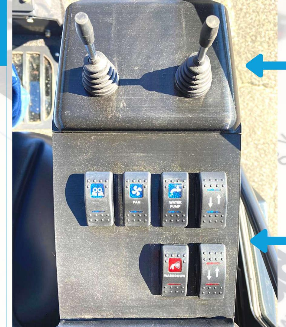
Fully independent left / right gutter broom joysticks
