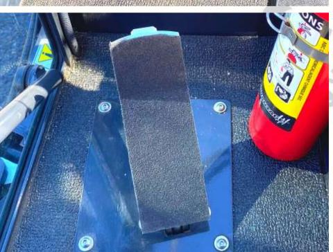
Hand parking brake - disc brakes on rear wheels
