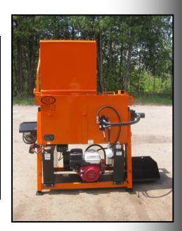
Each base unit includes a diesel burner system with flame out protection, a burner timer, and a hydraulic drive mixer which is driven from the truck's hydraulic system.
