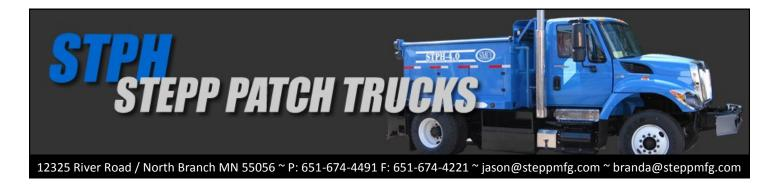
Stepp STPH Patch bodies have triple wall construction, inner hopper constructed of 10 gauge material. Oil jacketed chamber to be constructed of 12 gauge material insulated with 2" of 1½# density hi-temperature fiberglass insulation. Heat risers are designed into the hopper to help evenly distribute heat into the center of material. Insulation cover to be 16 gauge. Shall be mounted to the truck chassis with a spring loaded slip saddle mount.
