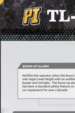
Notifies the operator when the boom is over legal travel height with an audible buzzer and red light. The boom-up alarm
