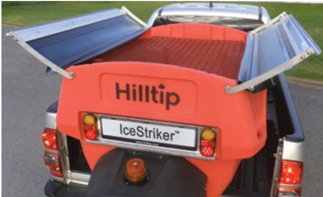
Two-piece tarp mechanism and top screen
