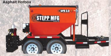
to heat the center, as well as the bottom and sides of the unit. Units requiring additional burners are not the answer due to the fact that you just need time, and the burner that is in the hot box is down fired for more consistent heat. Adding the additional burner is an additional maintenance and cost, a well designed hot box has heated surfaces in the center of the unit.
