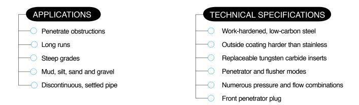
This egg-shaped nozzle is sure to get down the line and back again without hang-ups. With 8-degree, low-angle jets and front penetrating port, this sleek nozzle can easily get to some of the farthest blockages in need of removal. The EG Penetrator can also convert quickly to flushing mode by inserting its front plug.
