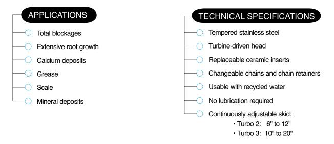
This innovative, highly reliable and efficient cutter offers superior drive and thrust to work through the toughest and hardest obstructions. The chain retainer is driven by a high-performance turbine that provides unsurpassed results in the removal of roots, grease and mineral deposits.
