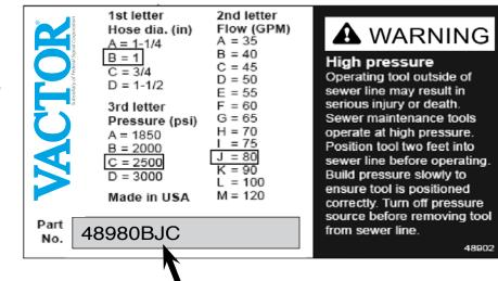
**Example**: If you want a Wedge nozzle on 1" hose at 80 GPM and 2500 PSI — the product chart above indicates part number 48980BJC would be the part to order.
