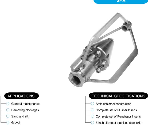
The low-angle jets and the rugged stainless steel construction of the JPX nozzle provide excellent penetration and flushing with a single, highly durable nozzle. This model is provided with a full package of inserts to quickly and easily change between penetration and flushing modes. Stainless steel skids surrounding the JPX body greatly reduce body wear to provide long-term performance.
