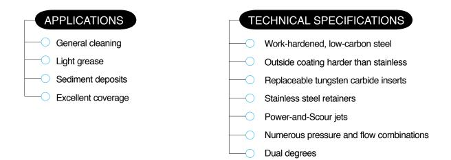
The Power Cleaner is an 8-jet nozzle with great coverage and cleaning ability. The rugged cone shape assists with forward travel while its power-maximizing internal cup diverts the jet spray backwards to flush out unwanted dirt and debris.
