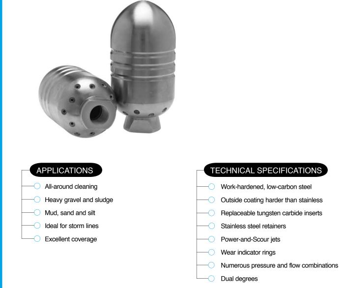
The Mad Flusher lives up to its name with its heavy-duty construction and powerful spray action. High-angle jets spray surrounding pipe walls quickly in large pipes, while low-angle jets propel debris down the line for maximized cleaning effectiveness. Indicator rings reveal when the nozzle body is fully worn and ready to be replaced.
