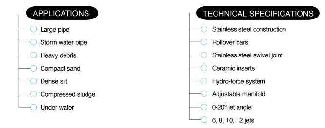
The HydroSurge<sup>™</sup> is the ultimate, high-performance cleaning nozzle for large pipe applications. The adjustable nozzle plate provides incredible traction and cleaning performance. The cleaning mode of 15 to 20 degrees removes heavy deposits from the bottom of the pipe.
