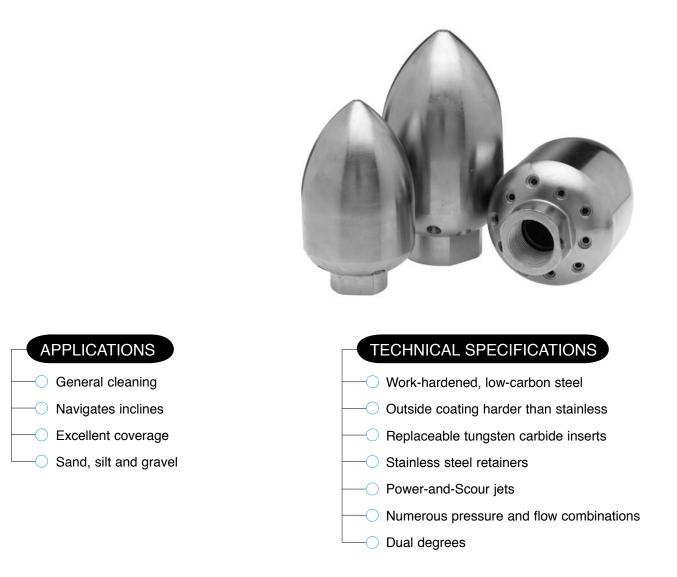
When your job requires high thrust and effective cleaning, this 10-jet nozzle gets the job done. The Super Flusher's rugged cone shape assists forward travel while its power-maximizing internal cup diverts the jet spray backwards to flush out loose obstructions and debris.
