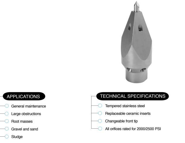
These Chisel nozzles provide excellent performance in difficult cleaning situations, especially when pipe deformations or total blockages are present. The different forward-jet options and sharp edges assure fast and reliable cleaning. Our chisel nozzles with forward jets and drill points penetrate deeply to remove and flush total blockages.
