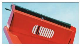
The dump body protects the truck cab, rear window and storage compartments. A roll-up nylon-reinforced lumite tarp that covers the entire load is available for TC-300 series bodies.
