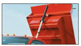
The TC-300 Series Hoist is a 6 ton, 3-stage telescopic type, powered by an electrohydraulic pump that can be used with automatic transmissions.
