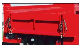
A super duty 18" double acting tailgate is hinged top and bottom for controlled spreading or complete clean dumping. The lever handle allows single-handed operation.
