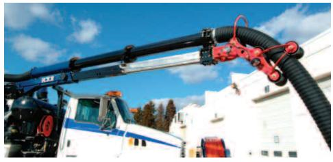
The new Vactor 5x5 boom telescopes outward five feet and allows the hose to move downward an additional five feet. Movement is controlled by a convenient wireless remote (optional).
