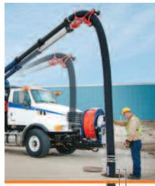
The new CB nozzle adds five feet of length to reach down into catch basins or sewer holes with ease.
