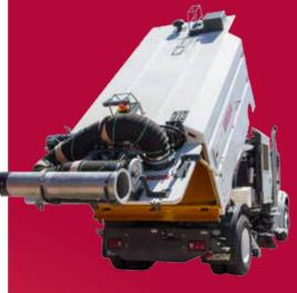
QUICK COMPLETE DUMPING 10 and 13 cubic yard (7.65 and 9.94 cubic meter) hoppers are constructed with 10-gauge steel walls and ceiling, a 1/4 inch (6.35 mm) thick floor with drop-down screens for quick cleanup.
