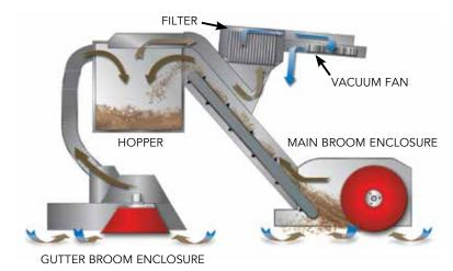
Elgin's filter is waterless dust suppression technology as patented - U.S. #7,281,296 B2, U.S. #6,584,157 B2.
