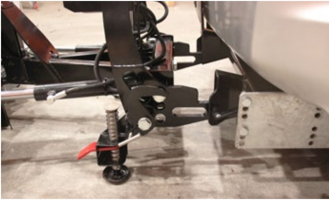
Quick hitch - lift shoe handle to attach your plow to the vehicle.
