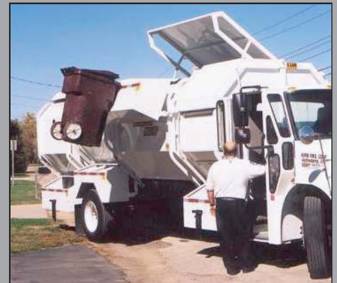
In addition to the troughs, the cart tipper option provides the ability to pick up carts.
