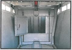
The Kann densifier wall (shown with access door open) is engineered to compact commodities to achieve maximum payloads
