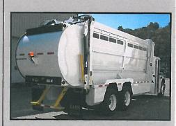
The Kann Up and Over Recycler equipped with a 5 yd<sup>3</sup> bubble tailgate option for added capacity.
