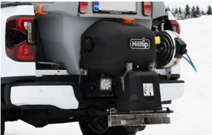
Beacon light (orange) & LED work light (white)
